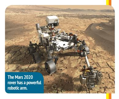
The rover's assortment of instruments includes a drill at the end of its robotic arm to dig for soil samples that astronauts will collect and bring back to Earth; an advanced camera system; **sensors** to test temperature, wind speed, and direction; and a high-tech X ray tool to analyze the chemical makeup of rocks at a fine scale.
