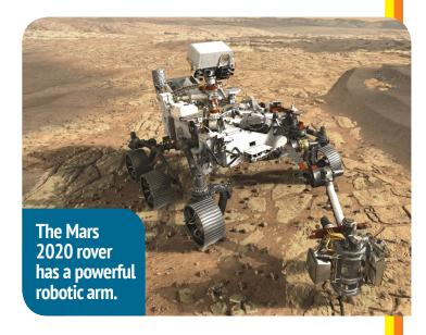
in the heavy dust and extreme cold on Mars. The arm also has a drill to dig for soil samples.
