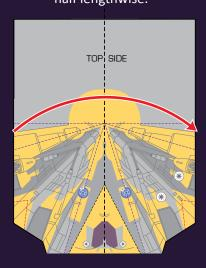
Find the blue triangle. Fold on the black dashed line that runs beside the triangle. Crease. Fold the other way. Unfold.
