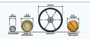
At 20 inches in diameter, Curiosity's wheels are much bigger than the wheels of previous rovers.
